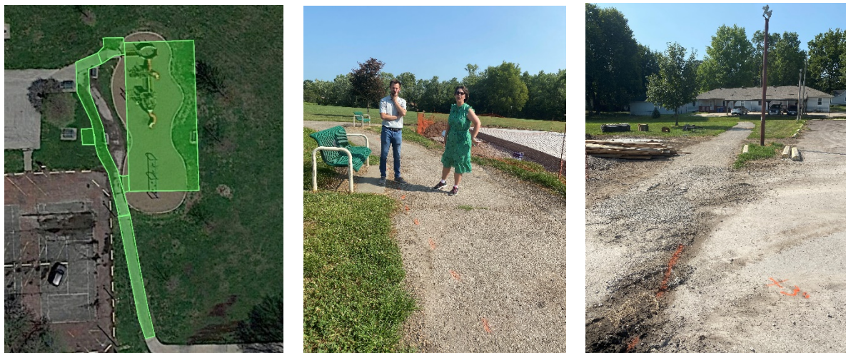
Proposed new sidewalk around Basket Ball Court . this will allow the backfill to be tapered to provide better drainage.
